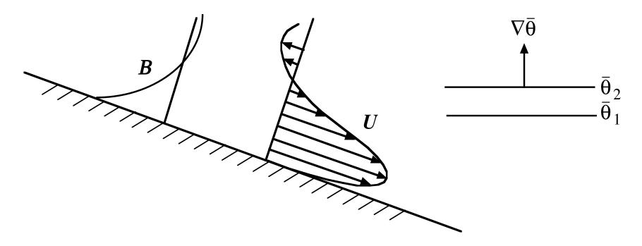
Steady 1-D flow of viscous fluid along a uniformly cooled sloping planar surface in a stably stratified atmosphere.
