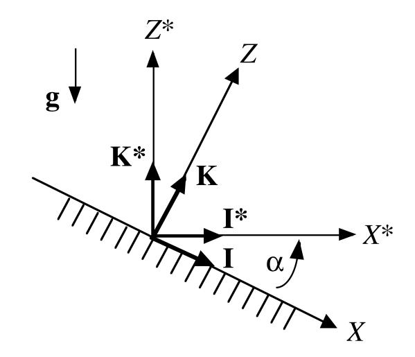
*X*, *Z*: along-slope and slope-normal coordinates, respectively.*U*, *W*: along-slope and slope-normal velocity components, respectively.
